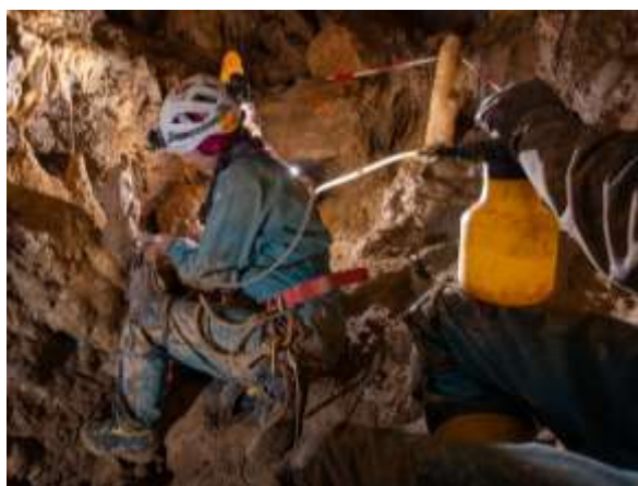
Figure 2: Sampling of a calcite core in a stalagmite with a hand-held drill and a water flushing unit.
