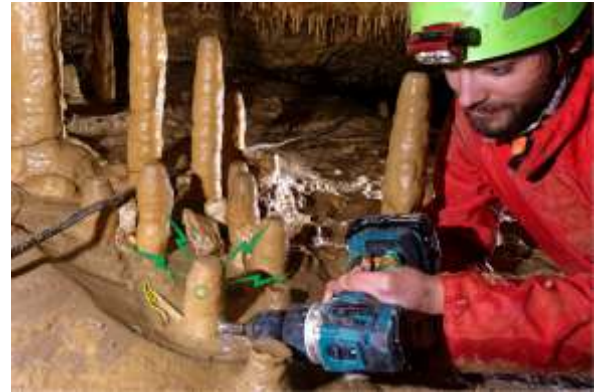
Figure 4: Micro-core drilling of the SANG 20-04 speleothem. Note the shocks (white dots in the green circle) showing the evacuation of the pebbles after growth.
