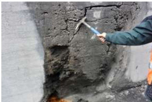
Figure 1. Ghost rock in the Gauthier-Wincqz Quarry in Soignies, Belgium. The limestone, a massive Tournaisian (Mississippian) 'encrinite' was partially dissolved, especially its micritic part. The larger remains of the crinoid fossils give a granular aspect to the 'ghost'. Inside the ghost-rock,
