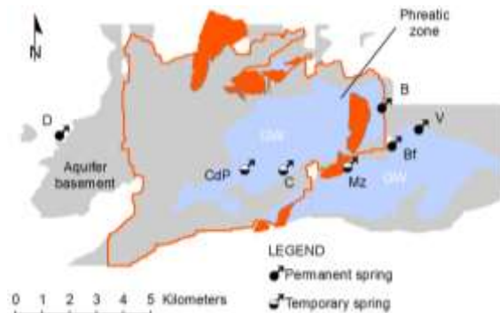
Figure 3: Delineation of the catchment area for the Beuchire-Creugenat karst system. Orange areas refer to allogenic parts and "GW" to the extension of the phreatic zone.
