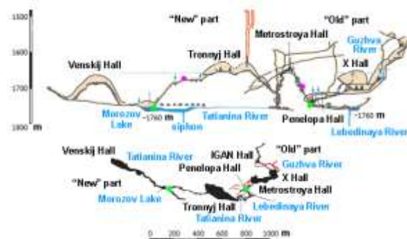
Figure 1: Profile and plan of the bottom part of the Snezhnaya cave system (from SHELEPIN et al. 2019) indicating the locations of the loggers. Places of levelloggers are marked by green circles, barologgers are by magenta circles (only on the profile).
