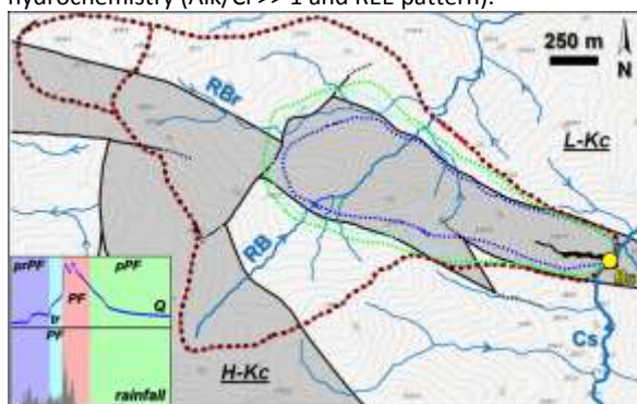
Figure 4: Bossea catchment drainage during the 2016 flood. The colored dashed lines mark the drained areas during the flood subsequent phases. The box reports the Mora creek hydrograph and the flood phases.
