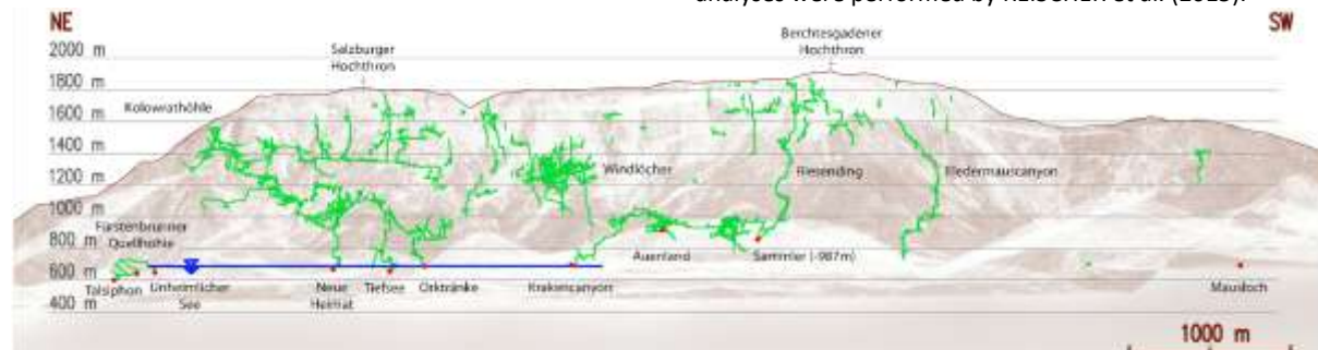
Figure 3: Cross section through Untersberg with major caves, logger positions are indicated by red dots (mod. from Zagler, 2016), the saturated zone by a blue line. Water level of the saturated zone may vary by 40 m at Unheimlicher See.
