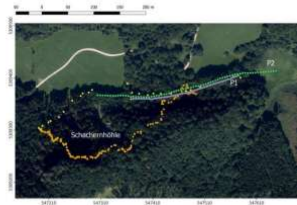
Figure 3: Overview of the surveys carried out: the resurvey of the Schachernhöhle is shown with orange and the geophysical profiles P1 with blue and P2 with green points. The survey connecting both measurements is shown with yellow points. Underlaid is an orthophoto of the region.
