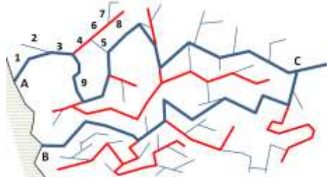
Figure 4: Example of order of surveyed cave segments.
