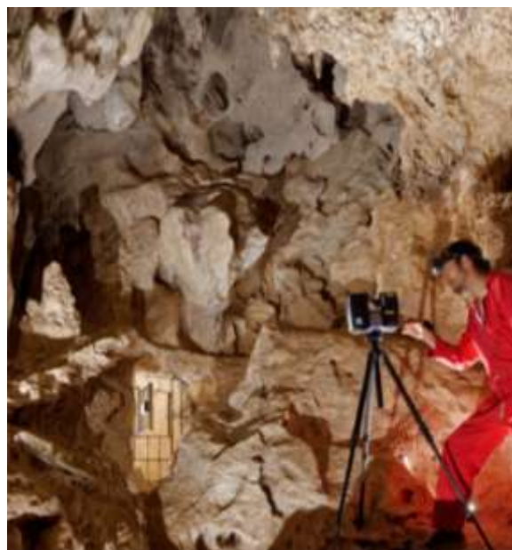
Figure 2: 3D survey in the Planchard cave (West of the Chauvet cave), with a Faro Focus 3D.
